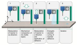
Figure 1: The Chemical Stitching process and its process steps
