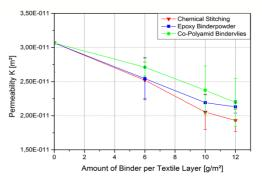
Figure 4: Permeability depending on binder system at 90° fiber orientation
