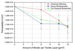
Figure 3: Permeability depending on binder system at 0° fiber orientation
