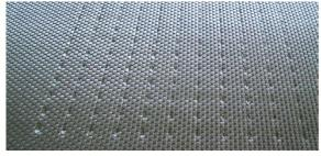
Figure 2: Preform locally fixed by using "Chemical Stitching" approach
